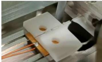
FIG. 2. Fiber cavity setup with mount (white) and piezoelement (yellow).
