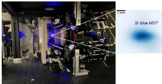
FIG. 1. Picture of the current state of our experiment, with a magneto optical trap (MOT) on the strontium-88 blue transition.
