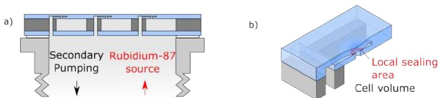
FIG. 1. *a)* A wafer of cells placed on a vacuum chamber to fill the cell with rubidium-87 *b)* Local sealing using a CO<sub>2</sub> laser.
