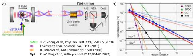
FIG. 1. a) An atom is trapped in an optical cavity and multiple laser beams drive Raman transitions, perform single qubit rotations and produce single photons. The photons are measured with a setup that can switch between two settings of the measurement basis. b) Scaling of the coincidence rate for a N-photon state. Our data are in blue (GHZ) and red (cluster).
