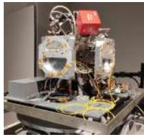
FIG. 1. The inertial sensor
